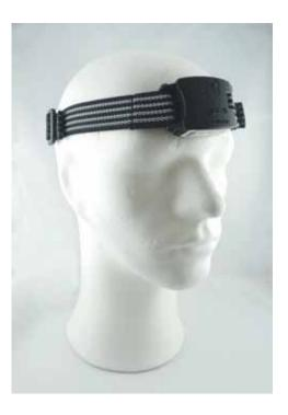
8. If necessary, correct the position of the HEG neuro housing on the forehead. It should be positioned centrally on the forehead. The sensor may be too tight or too loose. Then change the length of the straps again.
